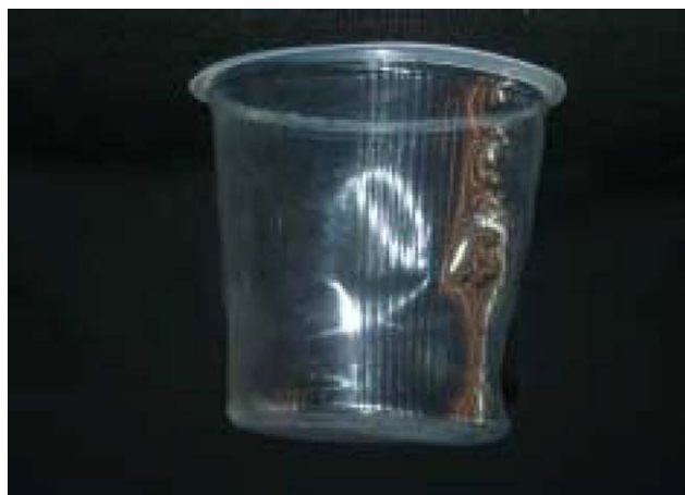
Fig. 2. The warpage of a polymeric product during its application.
